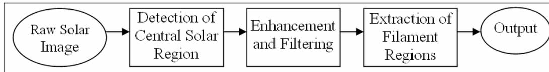
Figure 1. The major stages in the detection process
