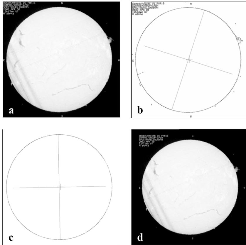
Figure 2. Limb fitting and image standardization stages; (a) original image, (b) initial ellipse fit, (c) refined ellipse fit (d) Standardized image after a geometrical correction. The small cross near the centre of (b) and (c) indicates the position of the initial estimate of the disk centre while the large cross indicates the orientation and centre of the ellipse fitted to the edge points in the figure.
