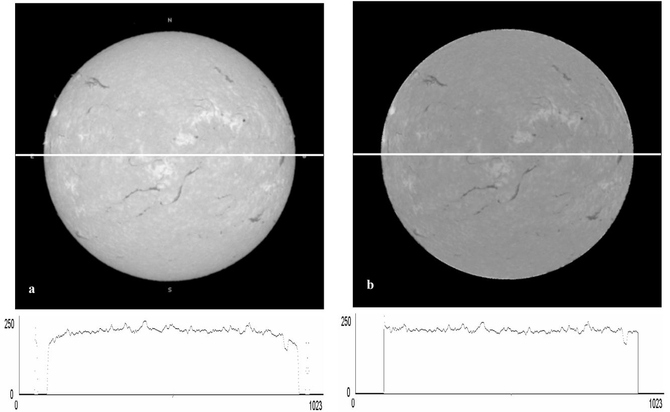
Figure 5. (a) Original H $\alpha$  image, (b) H $\alpha$  image corrected using median of rows of polar image, with plots of the intensities along the horizontal lines drawn through the images shown at the bottom.
